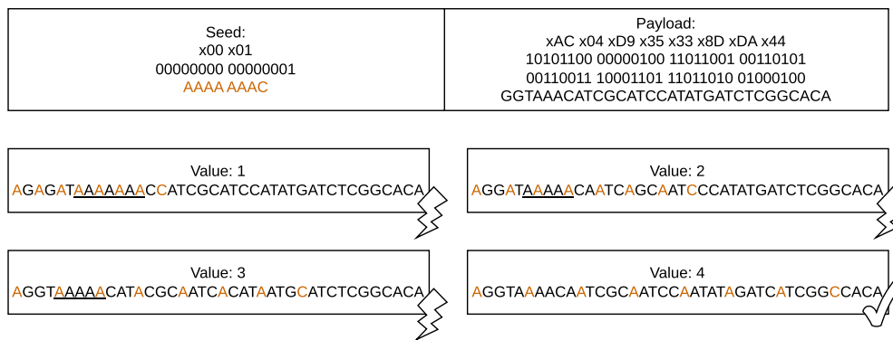
Fig. 2. Seed spacing with different interleaving values for a specific payload. Assuming a maximum allowed homopolymer length of 4, in the absence of interleaving, the reason for the rule violation is the seed itself. This method can be used both per byte and per base (i.e., nucleotide), offering fine-grained control over the interleaving process.
